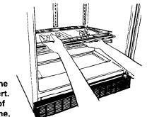
Remove the glass insert. Lift front of cover frame, then the back.
